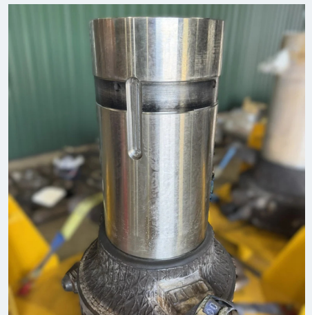
Cutter drum laserclad repair
